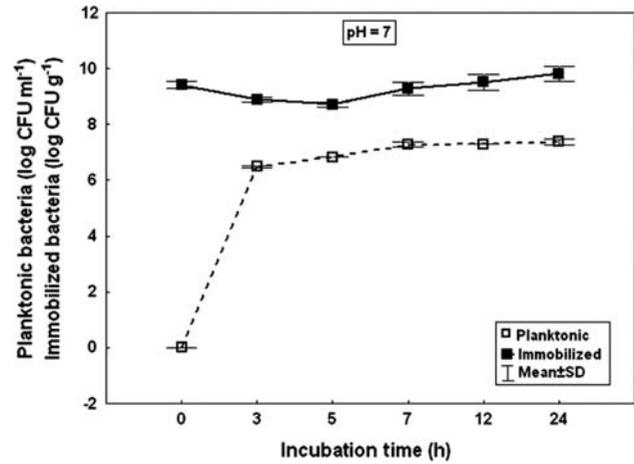
Figure 3. The density of planktonic and immobilized bacteria in the reactors with wastewater of initial pH 7, monitored for 24 h after the addition of bioparticles.
