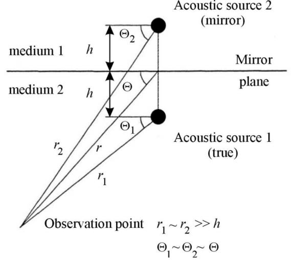
Figure 1: Acoustic dipole modelled by a virtual source
