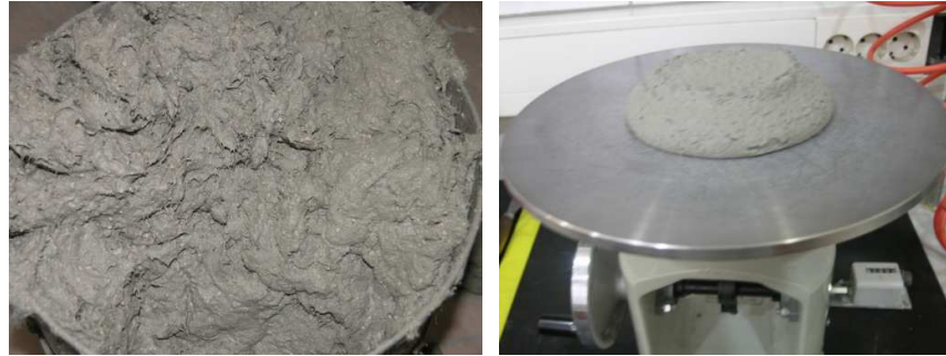
Figure 2: Fresh mortar with wool fibres and testing of consistence (flow table)
