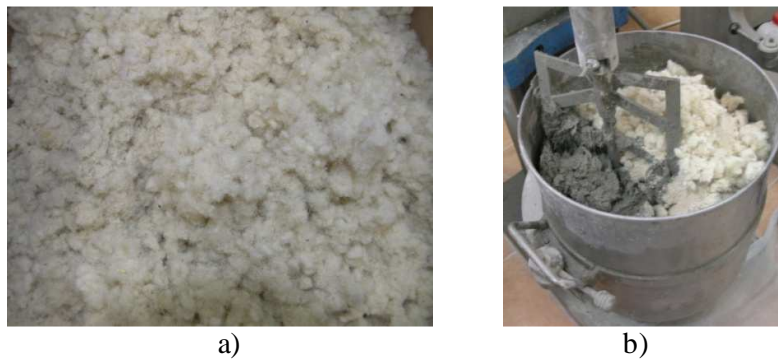
Figure 1: Sheep wool fibres and preparation of mortar
