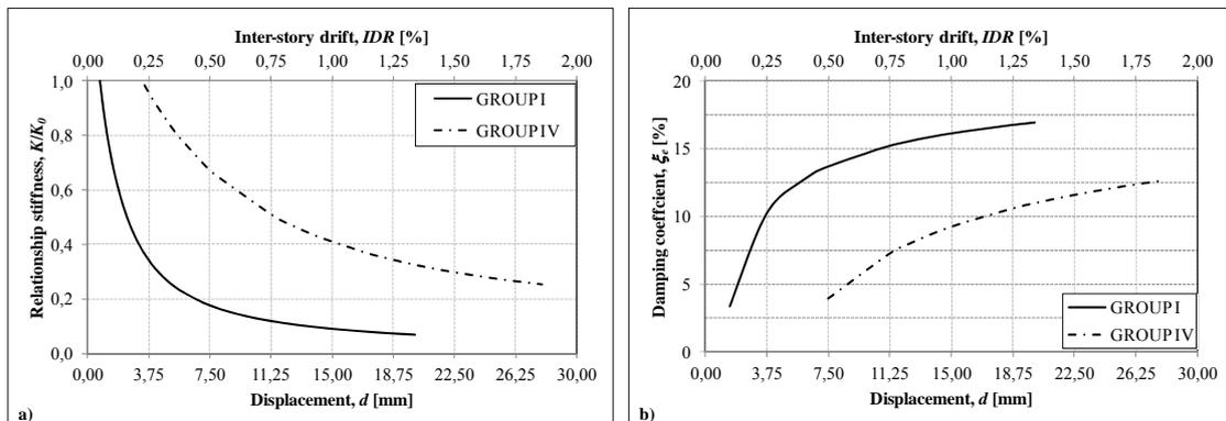
Figure 5. Stiffness degradation for all model structures and damping coefficient as a function of horizontal displacement (storey drift) levels
