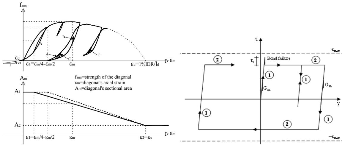
Figure 8. Hysteretic behaviour of the diagonal struts and variation of the area of the masonry strut
