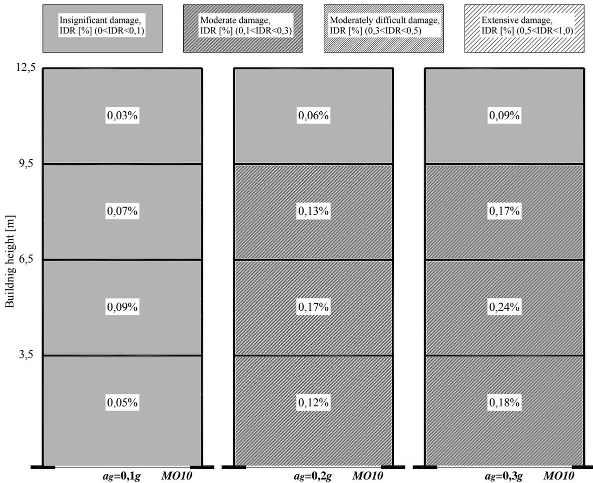
Figure 14. Infill wall's damage levels
