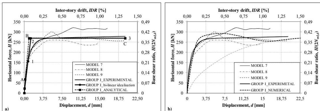
Figure 9. a) Comparison of experimental and analytical results b) Comparison of experimental and numerical results
