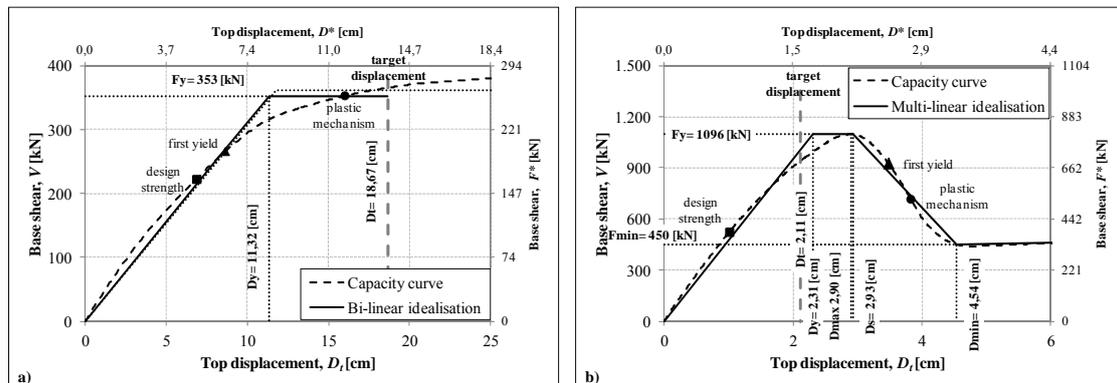
Figure 12. Pushover capacity curves and their multi-linear idealisations ( $a_g=0.3g$ )
