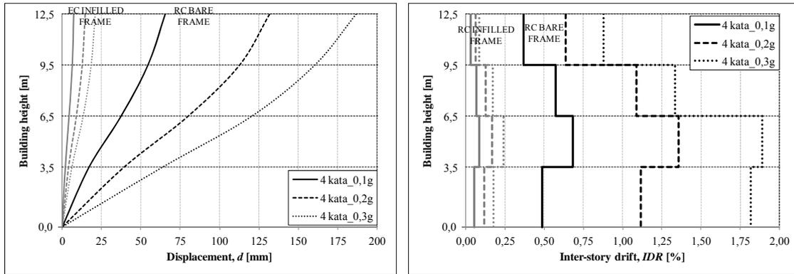
Figure 13. Horizontal displacements and inter-story drifts for the target displacement
