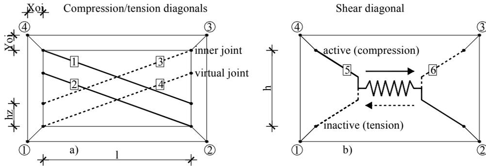
Figure 7. Inelastic panel element, a) compression/tension diagonals, b) shear diagonal
