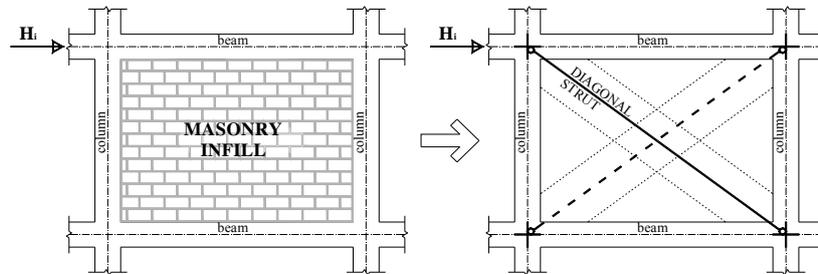
Figure 6. Macro-model using equivalent diagonal strut
