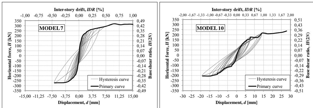
Figure 2. Lateral load – displacement curves of the representative RC infilled specimen of GROUP I and of the RC bare frame model GROUP IV
