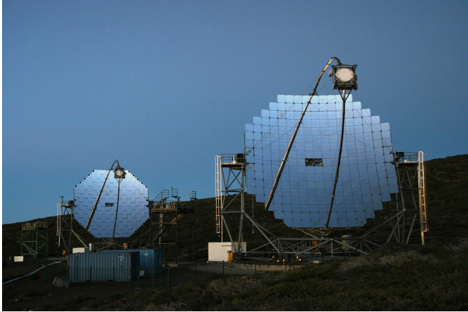
Figure 1: The two 17 m diameter MAGIC telescope system operating at the Roque de los Muchachos observatory in La Palma. The front telescope is MAGIC-II.
