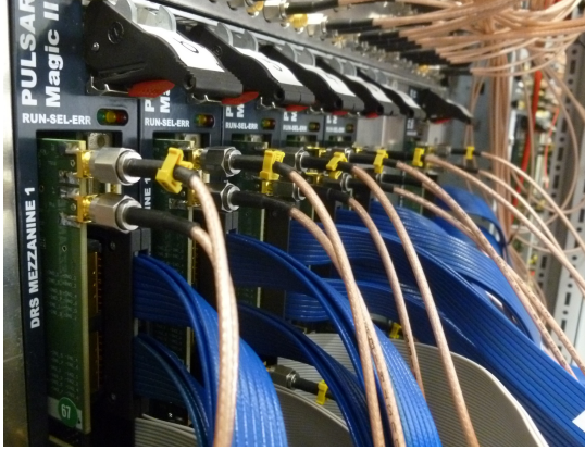
Figure 6: A close-up into the electronics, which read out the ultrafast signals produced by the Cherenkov photons from cosmic-ray induced atmospheric showers in the camera of the MAGIC telescopes. The DRS4 mezzanines (the green cards hosted by the PULSAR motherboards) are connected to the receiver boards by means of 24-differential-lines analog cables (blue) and synchronized by two SMA cables (one for the trigger signal and one for the common reference clock signal).
