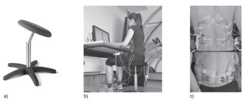
Figure 1: Representation of a) a novel chair with unstable seat (Active Chair®), b) a computerized office task while measuring EMG activity on the Active Chair® and c) EMG electrodes positions for left and right lower trapezius and erector spinae (upper picture) and rectus abdominis and obliquus externus (lower picture) muscles.
