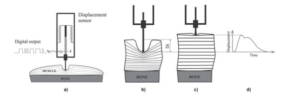
Figure 1: The principles of tensiomyographic measurement: linear displacement sensor (a) is pressed against the resting muscle (b) and during twitch muscle contraction muscle belly thickens and vertically presses the displacement rod (c) to measure a mechanical twitch response (d) (Adopted from previous publication of Šimunič, with permission).
