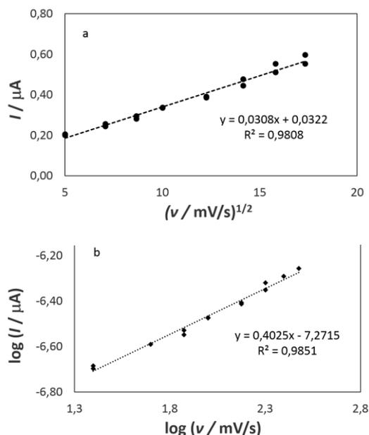
**Figure 4.** a) Anodic peak current,  $I$ , as a function of the square root of scan rate,  $v^{1/2}$ , b) Logarithm of anodic peak current,  $\log I$  as a function of logarithm of scan rate,  $\log v$ , at a glassy carbon electrode in solution of the title compound ( $c = 8.4 \cdot 10^{-5} \text{ mol dm}^{-3}$ ,  $I_c = 0.1 \text{ M LiCl}$  in DMF).
