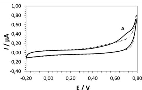
**Figure 2.** Cyclic voltammogram of the title compound ( $c = 1.1 \cdot 10^{-4} \text{ mol dm}^{-3}$ ) at a glassy carbon electrode ( $I_c = 0.1 \text{ M LiCl}$  in DMF). Scan rate: 100  $\text{mV/s}$ . a) 0.1 M LiCl (supporting electrolyte), dashed line and b) title compound, solid line.
