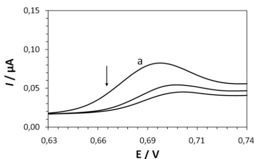
**Figure 5.** Differential pulse voltammogram of the title compound ( $c = 1.1 \cdot 10^{-4} \text{ mol dm}^{-3}$ ) at a glassy carbon electrode ( $I_c = 0.1 \text{ M LiCl}$  in DMF). Scan rate: 5 mV/s. First scan (a).
