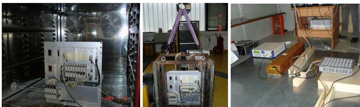
Figure 2.5: Environmental, shock and vibration immunity and electromagnetic compatibility tests of proprietary embedded control systems, [7]
