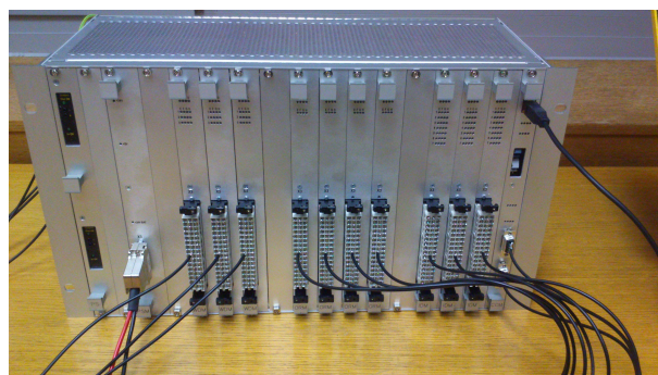
Figure 8.2: Safety platform mounting rack with installed electronic modules
