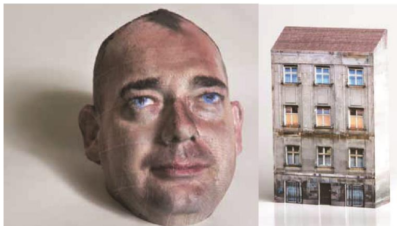
Figure 12: Photorealistic 3D model printed by Mcor Iris 3D Color printer technology
