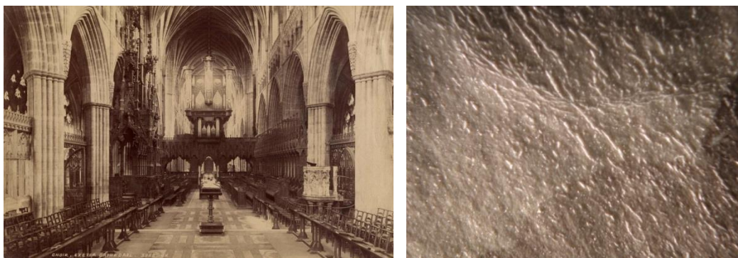
Figure 3: Original albumen print and microphotography showing cracking of light-sensitive layer
