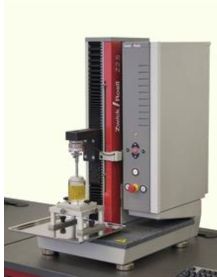
Figure 4: Zwick/Roell BDO-FBO 0.5 TS Tensile strength measuring device
