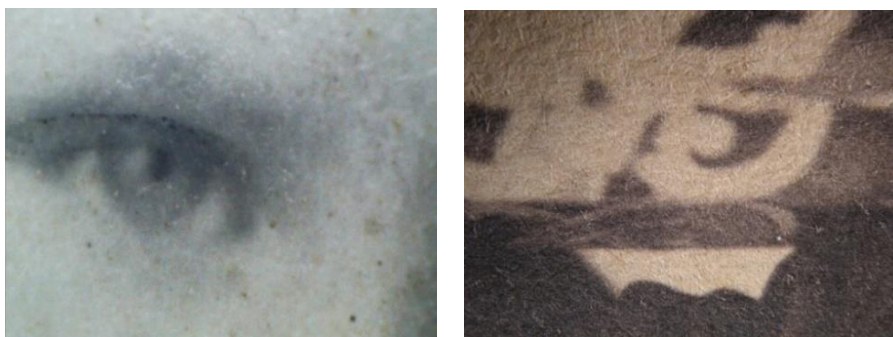
Figure 1: Microphotography of salted paper print (magnification 20x)
