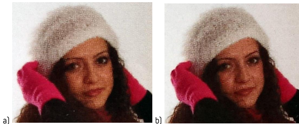
Figure 7. Details on reproduction: a) 200 lpi - 225dpi, b) 200 lpi - 400 dpi
