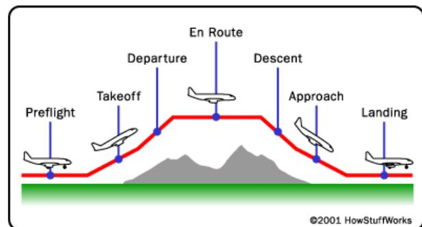
Fig. 2. Phases of flight [13].
