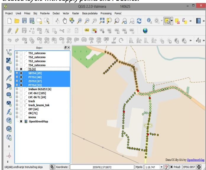
**Figure 5.** Newly created layers with supply points and PL zones
