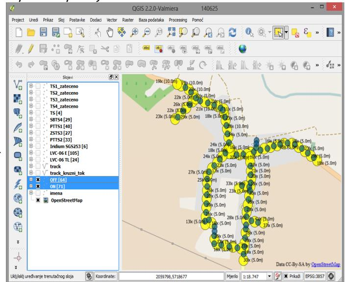
**Figure 6.** Layers with illumination measurement data
