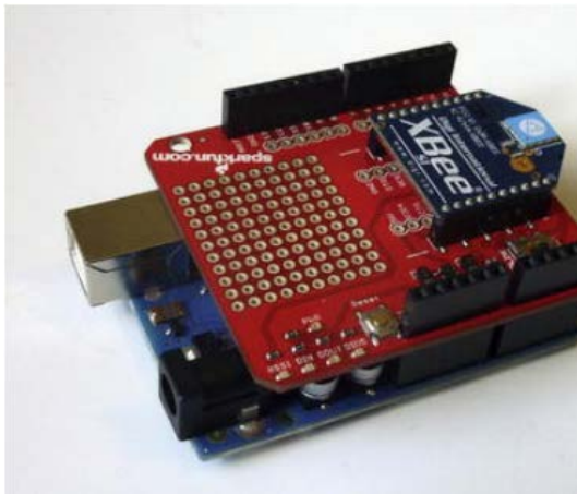
Fig. 2. An example of an upgrade (shield) of Arduino board
