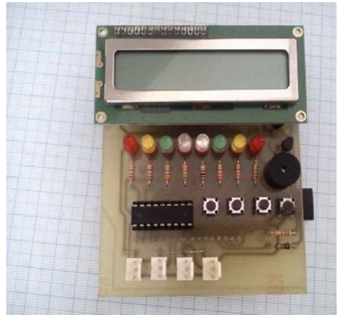
Fig. 3. LCD and LED expansion module created as DIY
