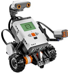
Fig. 1. Mobile robot with ultrasonic distance sensor or light sensor.
