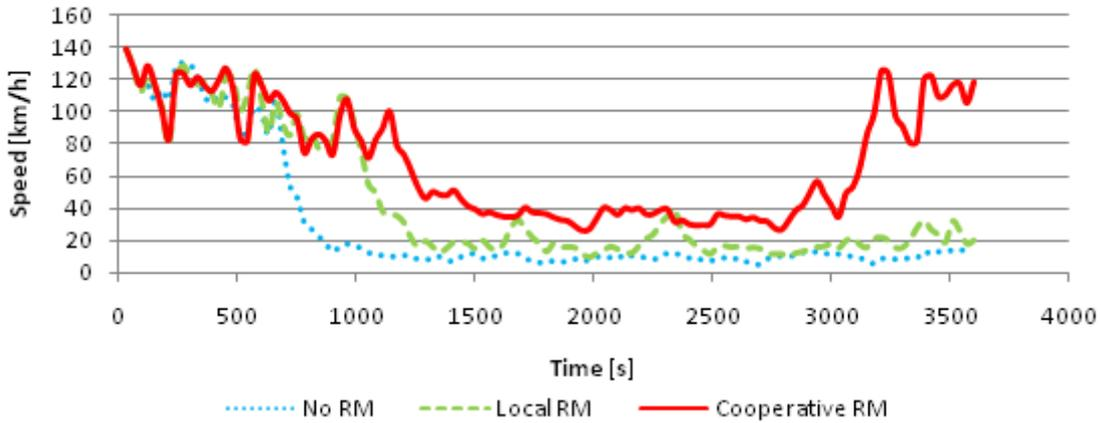
Figure 8 – Slow lane speed for the first segment
