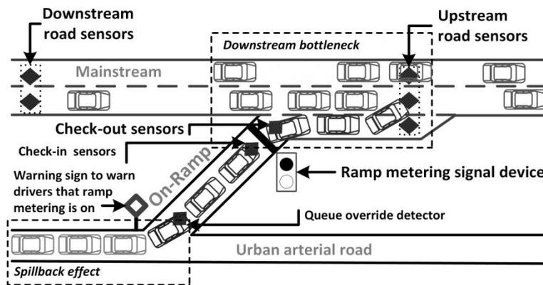
Figure 1 - Illustration of potential problems near an on-ramp [4]
