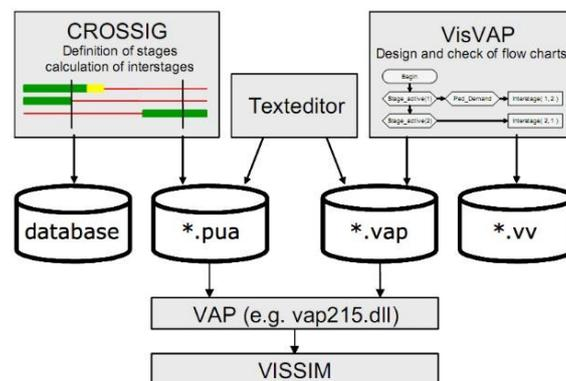
Figure 4 – Components of the VisVAP module [8]
