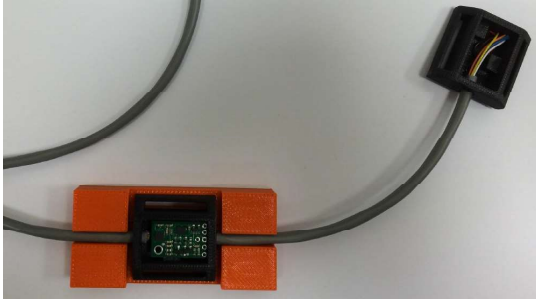
Fig. 4. DiverNet sensor node construction with daisy-chain wiring topology
