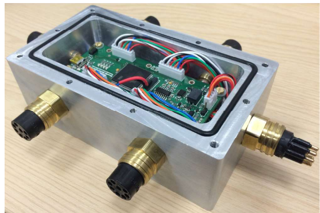
Fig. 2. DiverNet hub mechanical construction: Aluminium 5083 housing with main processing PCB and micro SubConn interface connectors
