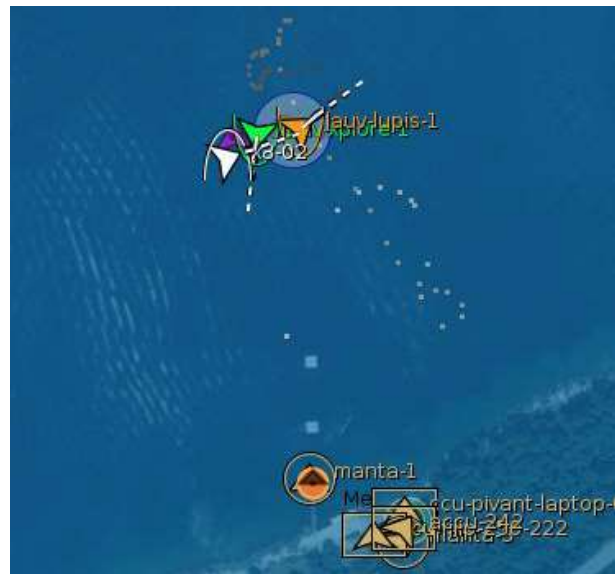
Fig. 11: Real-time visualisation of the heterogeneous system agents from Fig. 10 on Neptus, Decision Support System. Image shows 3 AUVs (orange, green and purple), UAV (white), and base station (brown)
