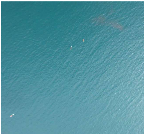
Fig. 10: Image from the UAV showing part of the Rhodamine WT patch and 3 AUVs on the surface, resting and transferring mission log data to the UAV
