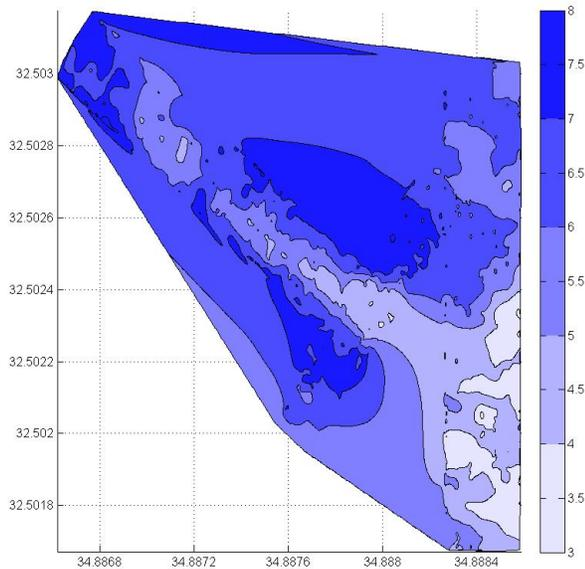
Fig. 7: Partial bathymetry map of the southern breakwater in Caesarea's outer harbor.
