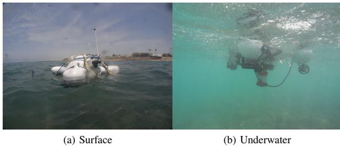
Fig. 2: The Pladypos operating at sea from two perspectives.
