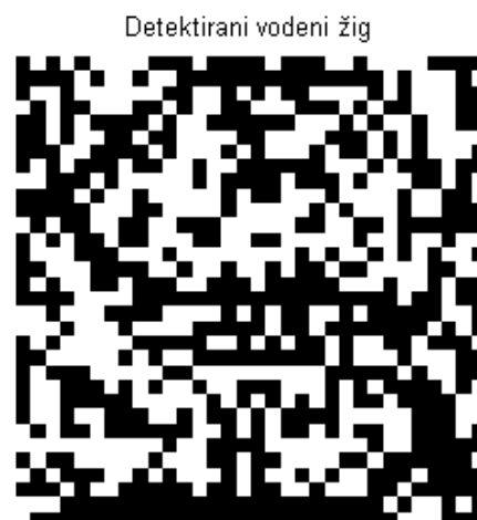
Slika 5.41 Gaussov šum ( \mu = 0.4 , \sigma = 0.01 ), gain=5
