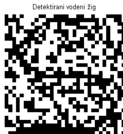
Slika 5.41 Gaussov šum ( \mu = 0.4 , \sigma = 0.01 ), gain=5
