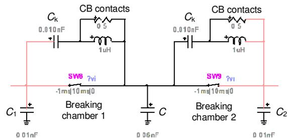
Fig. 7. Model of SF<sub>6</sub> circuit breaker with two braking chambers
