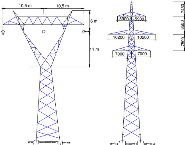
Fig. 4. Towers of the transmission line TL1
