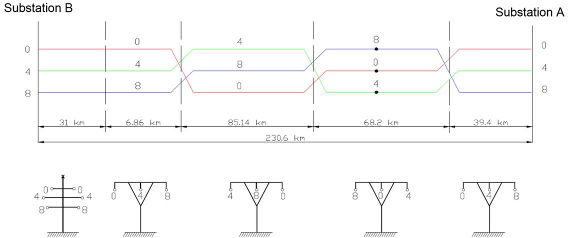
Fig. 3. Transpositions on 400 kV transmission line TL2
