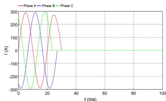
Fig. 9. Currents when switching off unloaded transmission line TL2
