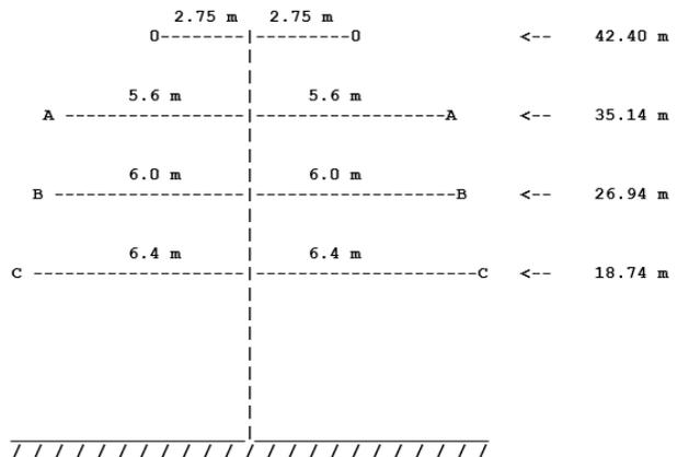
Fig. 6. Position of conductors at towers and their average heights (second section of transmission line 69.972 km)
