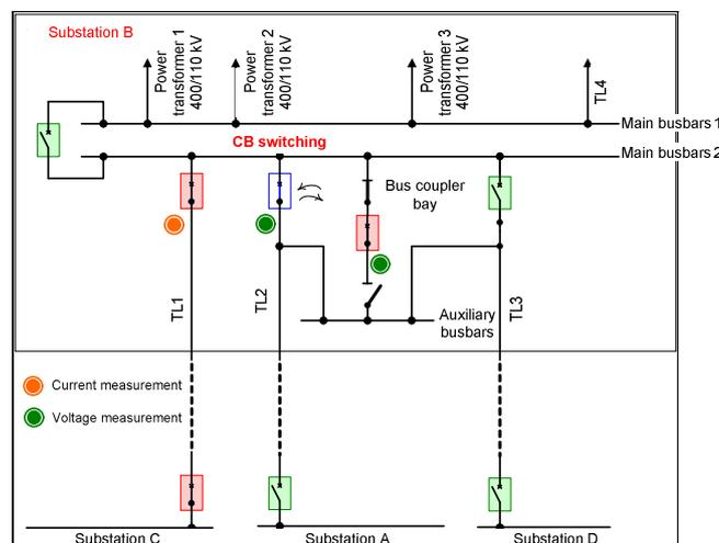
Fig. 2. Configuration 2: Testing of circuit breaker in 400 kV line bay TL2 when switching unloaded transmission lines TL2 and TL3
