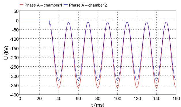
Fig. 13. Distribution of TRV across breaking chambers in phase A (with grading capacitors)
