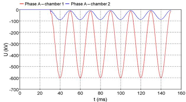
Fig. 12. Distribution of TRV across breaking chambers in phase A (without grading capacitors)
