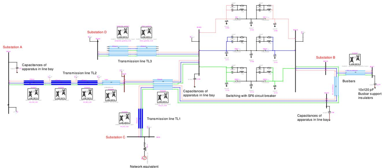
Fig. 8. EMTP-RV model of the of 400 kV transmission network
