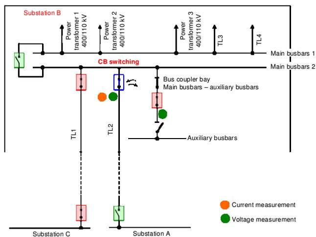
Fig. 1. Test configuration 1: Testing of circuit breaker in 400 kV line bay TL2 when switching unloaded transmission line TL2
