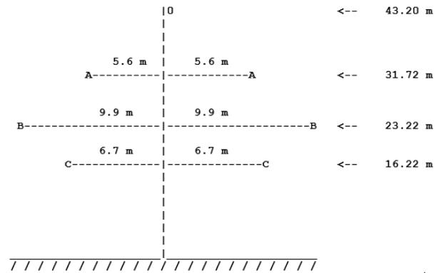
Fig. 5. Position of conductors at towers and their average heights (first section of transmission line 97.798 km)
