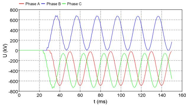
Fig. 11. TRV on CB without grading capacitors
