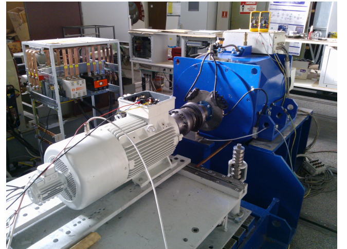
Fig. 8: 100 kW prototype and 450 kW load machine
