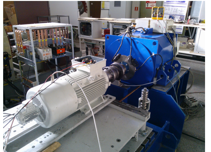
Fig. 8: 100 kW prototype and 450 kW load machine
