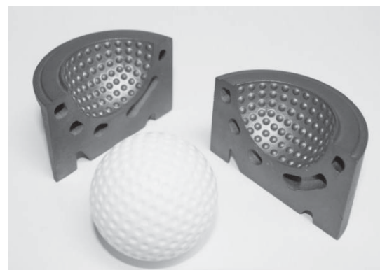
Figure 3. Mold for making golf balls produced by Direct Metal Laser Sintering process[1]
