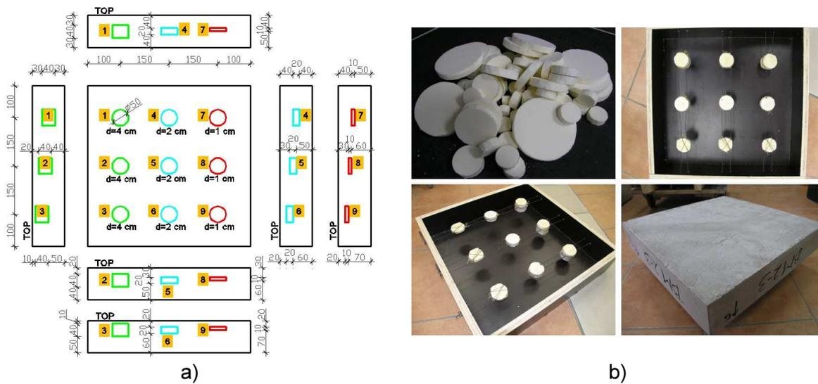
Figure 2: a) Schematics of the specimens BM x-2, dimensions in mm, b) photographs of the concrete test specimens with polystyrene defects
