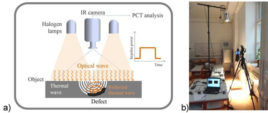
Figure 1: Thermal excitation of the object under examination using IRT: a) schematic representation, b) photo of the test setup
