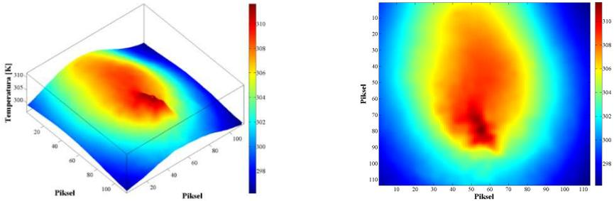
Figure 3: Optimal thermograms of selected specimen configurations, BM 2-2 bottom surface, distance 1.5 m, 3D and 2D representation
