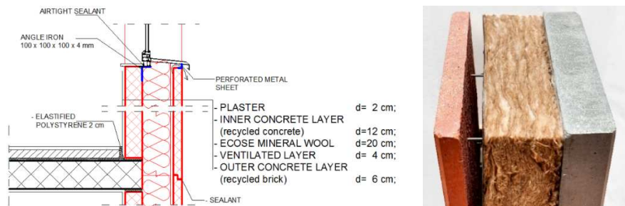
Figure 1: Composition of ECO-SANDWICH ® wall panel
