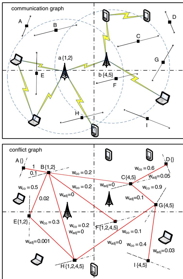
**Fig. 2** Communication and conflict graph illustration. The figure shows example of dynamic spectrum access scenario with corresponding communication and conflict graph
