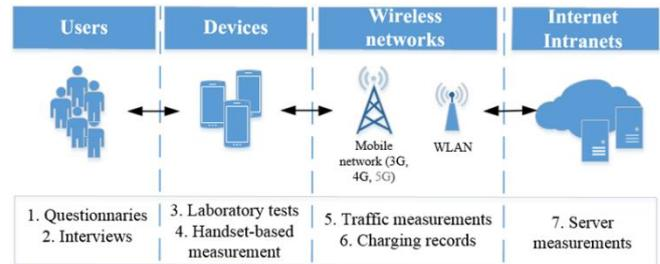
**Figure 2:** Sources for information and classification of research methods for data traffic measurement, [1], [9], [28]
