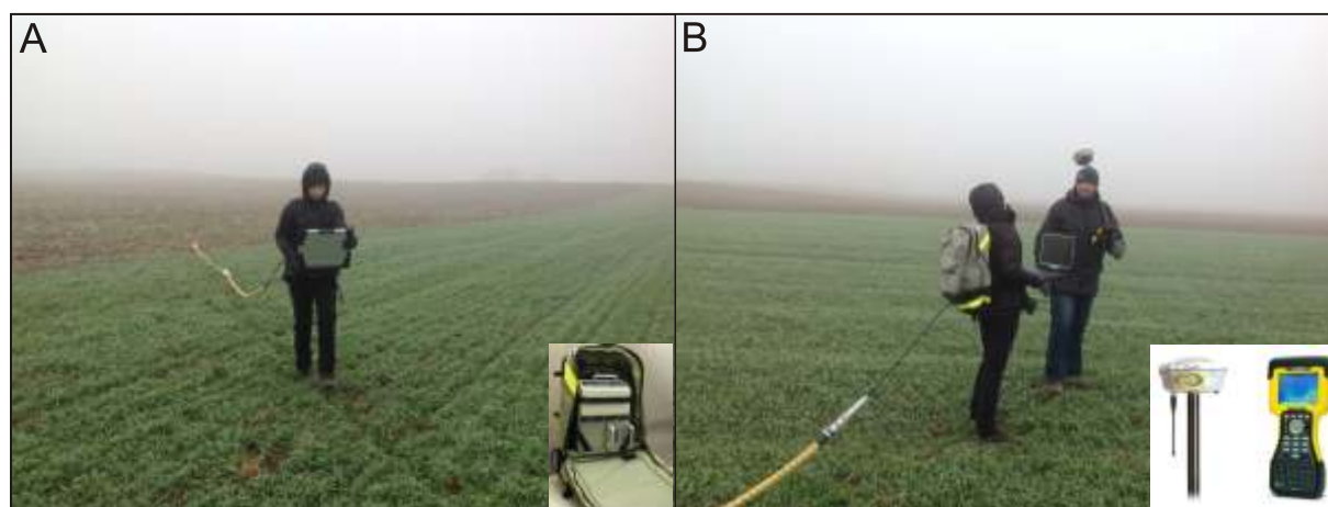
Fig. 8A – backpack-mounted acquisition system Malá ProEx GPR unit coupled with “snake-like” unshielded 50 MHz rough terrain antenna used in this study; B – the continuous GPS positioning along the surveyed GPR sections was achieved with the Trimble R8 GNSS Surveying System, with vertical and horizontal accuracy in the range of a few centimetres (see Marjanović, 2010; Marjanović and Link, 2011 for details)
