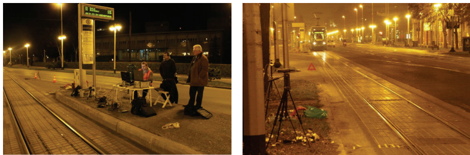
FIGURE 13: Conducting noise and vibration measurements under TMK 2266 pass-by at 30 km/h.
