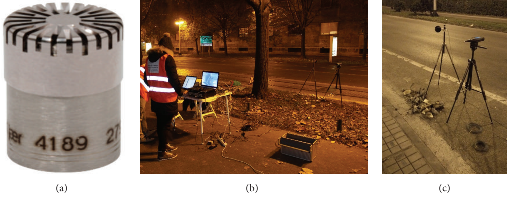
FIGURE 15: Microphone used for noise measurements (a); data acquisition and microphone positioning on different test sections (b and c).
