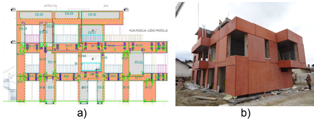
Figure 2. EC ® house: a) Position plan for southern façade; b) Construction site in March 2016
