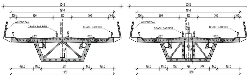
Figure 6. Multi-span semi-integral extradosed bridge – deck cross-sections; not suspended (left), suspended (right).
