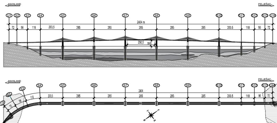
Figure 5. Multi-span semi-integral extradosed bridge – longitudinal layout and ground plan.
