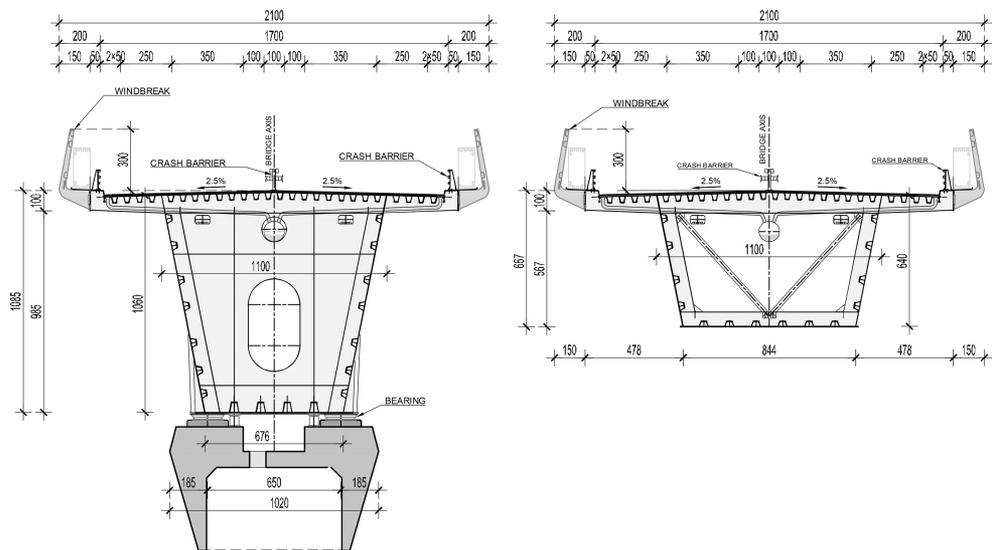
Figure 3. Box girder bridge – deck cross section above main span piers (left) typical deck cross-section (right).
