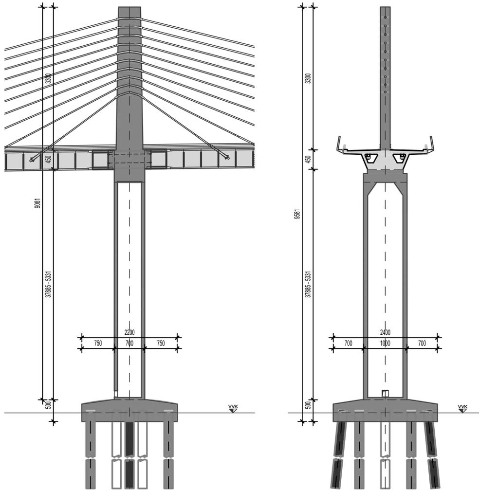
Figure 7. Pylons: Longitudinal section (left), Cross section (right).
