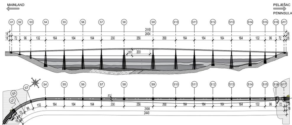
Figure 2. Continuous steel box girder bridge – longitudinal layout and ground plan.
