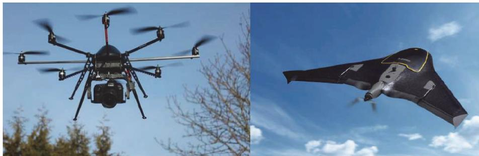
**Figure 1.1** Example of Multirotor (left) and Fixed wing aircraft (right)
