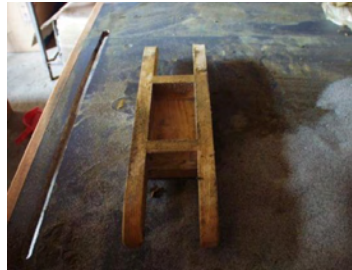
Figure 3 Mould for handmade bricks
