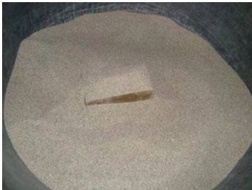
Figure 4 Sand-coating of newly made bricks
