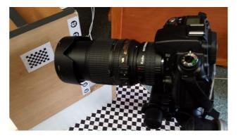
Figure 1. Camera with extension tube at the calibration field
