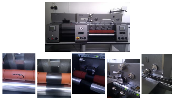
Figure 2: Prüfbau laboratory printing process, which simulates offset printing process
