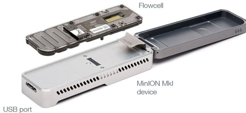
**Figure 1.1:** MinION Mk1 device illustration[8].
