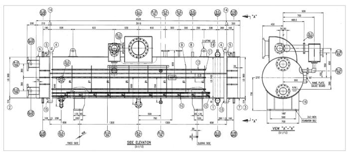
Figure 1 Overall dimensions and cross section of the analyzed low-pressure feed water heater
