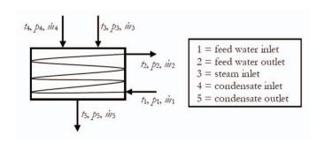
Figure 2 Low-pressure feed water heater symbol and operating parameters used in the numerical model
