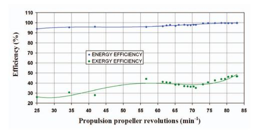
Figure 3 Energy and exergy efficiency change of low-pressure feed water heater
