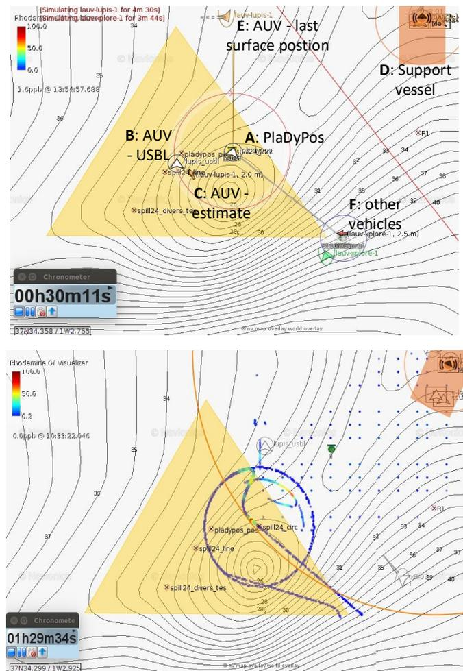
Fig. 10: NEPTUS visualisation, control and decision support software. Upper image presents position of the vehicles: A - position of the USV, B - AUV position from USBL, C - Neptus estimation/simulation of the AUV position, D - support vessel, E - last AUV surface position, F - position of another vehicle in the experimental arena. Lower image presents color map representation of the measurements. Source: LSTS Universidade do Porto.
