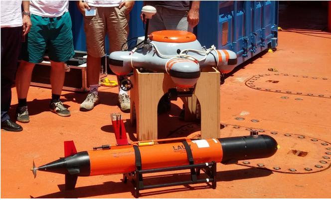
Fig. 2: AUV (orange vehicle at the bottom of the image) and USV used during the experiments in Cartagena.
