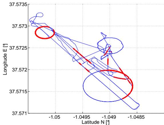
Fig. 11: Spatial concentration measurement during the series of consecutive missions initiated top side and replanned by the AUV supervisory system. Red dots indicate positive detection of the pollutant.
