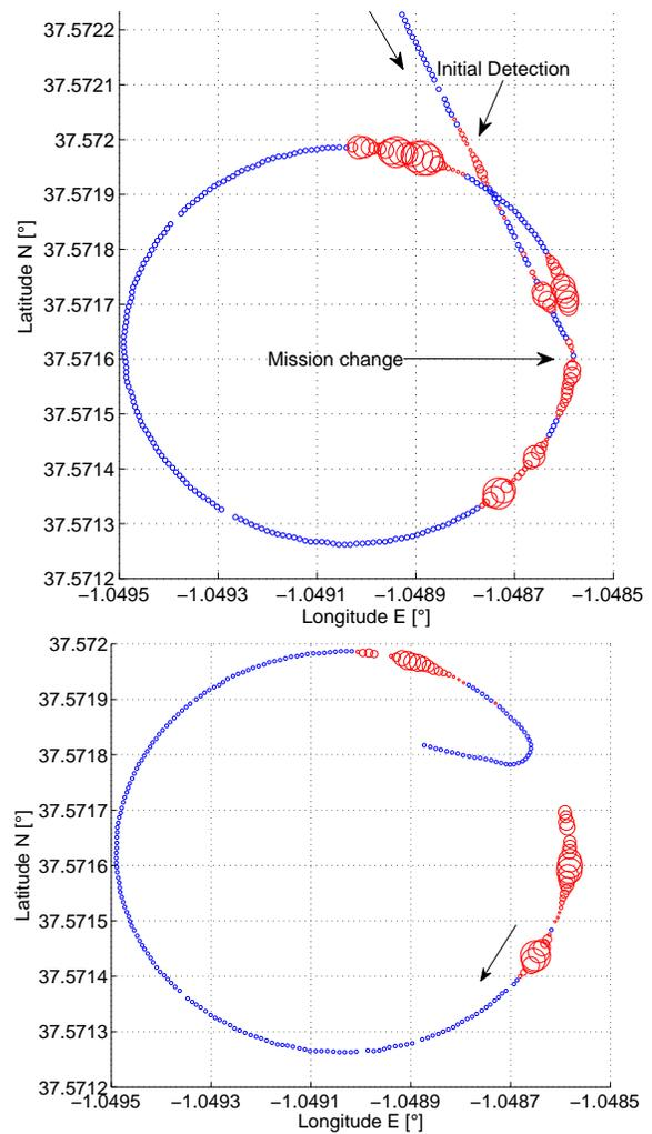
Fig. 8: Mission change and spatial concentration measurement during the two consecutive passages over the same area. Red circle indicates positive detection of the pollution. The size of the circle is proportional to the concentration measurement.
