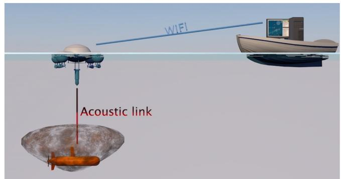
Fig. 1: Human-on-the-loop system. AUV (via USV) continuously feeds the operator with measurements through acoustic and WiFi links. Using the same links in the opposite direction the operator is able to abort or change the AUV mission or request some specific data.
