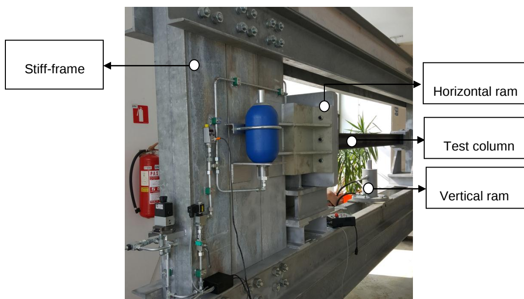
Figure 3: Column test facility at University of Split, Faculty of Civil Engineering, Architecture and Geodesy
