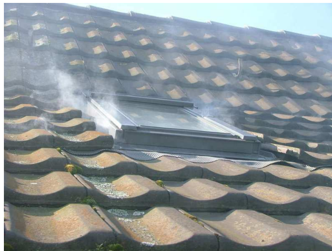
Smoke pressed out by a Blower Door fan to show the roof leaks
