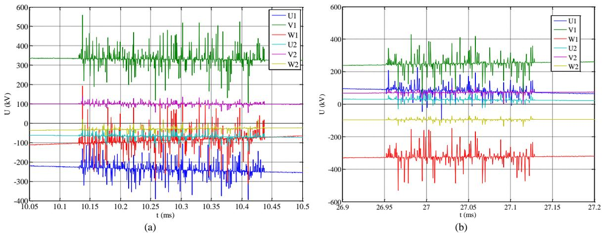
Fig. 16. Detailed overview of recorded overvoltages shown in Fig. 15: (a) first recorded overvoltage; (b) second recorded overvoltage
