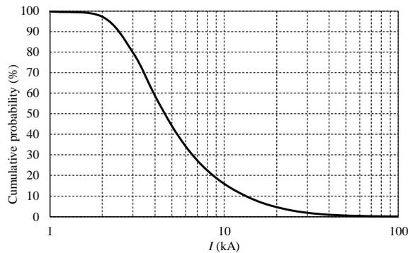
Fig. 18. Cumulative amplitude distribution of CG lightning strokes
