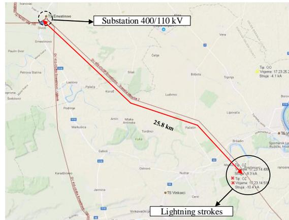
Fig. 20. Lightning strokes that probably caused lightning overvoltages recorded on the power transformer
