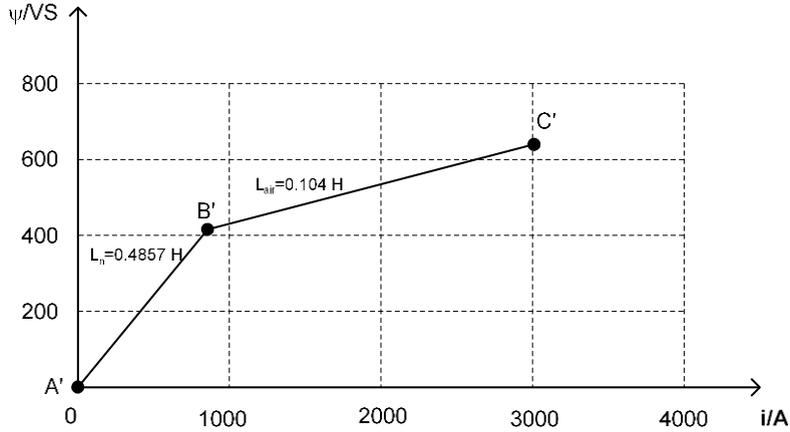
Fig. 3. Instantaneous flux-current saturation curve of shunt reactor
