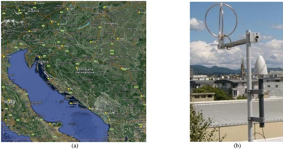
Fig. 14. (a) LINET sensors in Croatia and its neighbouring countries; (b) field antenna and a GPS receiver
