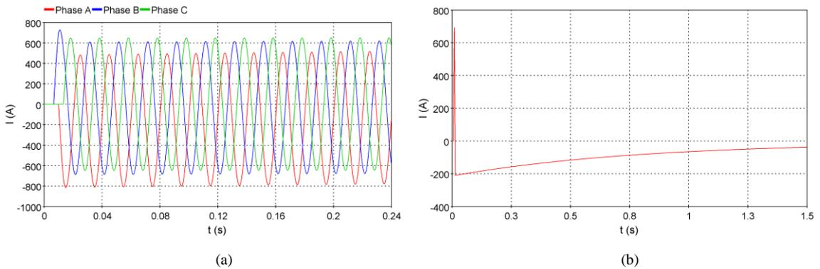
Fig. 8. (a) Inrush currents:  $I_{Amax} = -816$  A (1.23 p.u.); (b) zero-sequence current,  $I_{max} = 693.2$  A (1.05 p.u.)
