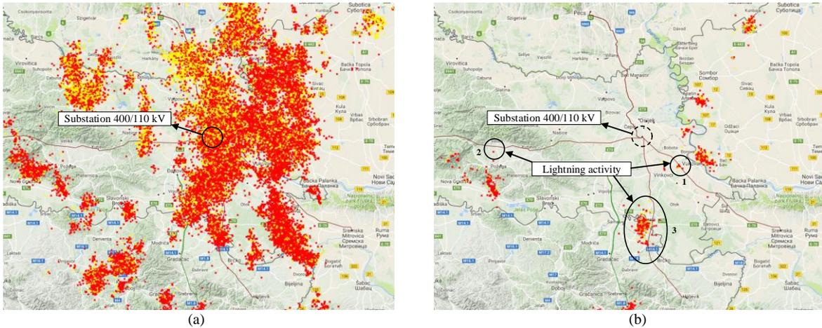
Fig. 19. Lightning activity in the vicinity of 400/110 kV substation: (a) time period  $\pm 3$  hours; (b) time period  $\pm 15$  minutes
