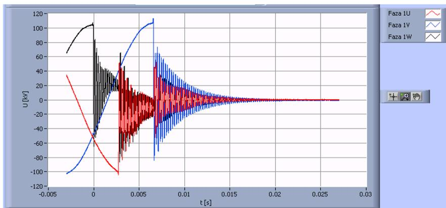
Fig. 11. Switching overvoltages recorded during controlled deenergization of shunt reactor
