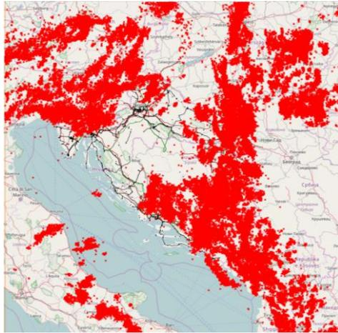
Fig. 17. Lightning activity (CG strokes) in Croatia and neighboring countries for the day in which overvoltages were recorded
