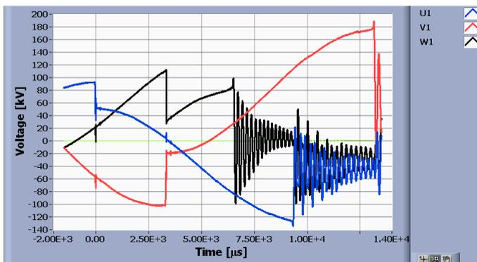
Fig. 12. Switching overvoltages recorded during uncontrolled deenergization of shunt reactor
