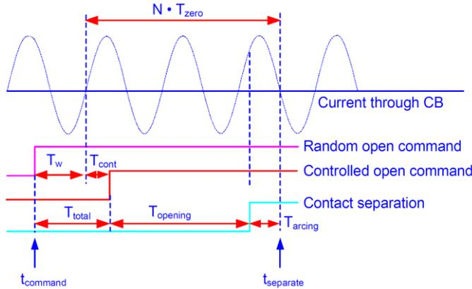
Fig. 10. Controlled opening sequence
