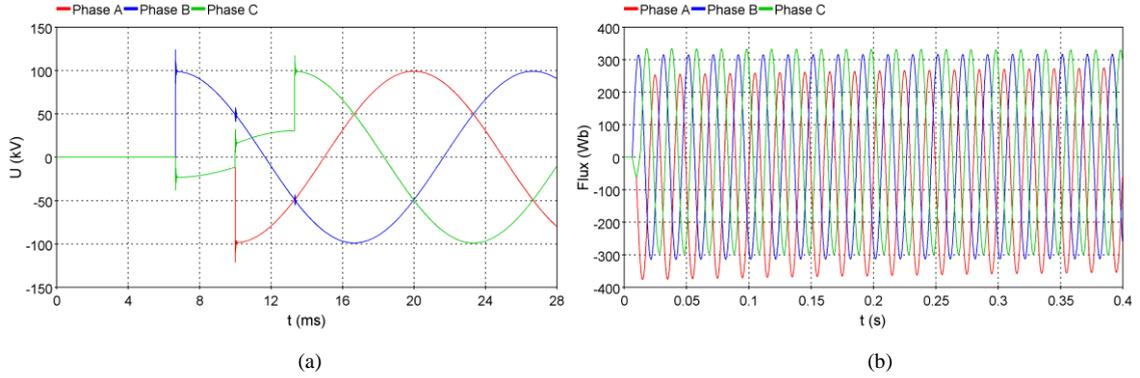
Fig. 7. (a) Shunt reactor voltages; (b) magnetic flux.
