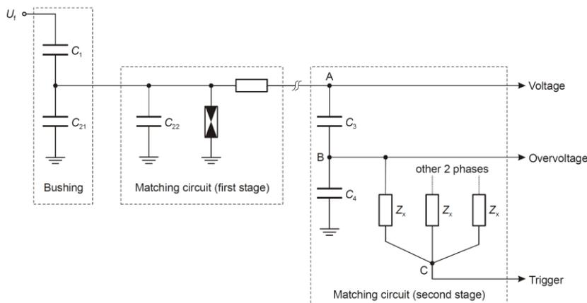
Fig. 2. Scheme of matching circuit
