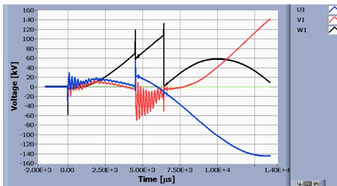
Fig. 13. Switching overvoltages recorded during uncontrolled energization of shunt reactor
