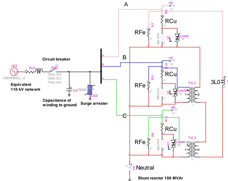
Fig. 4. Model in EMTP-RV
