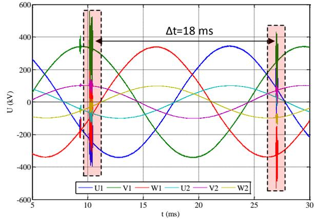
Fig. 15. Overvoltages recorded on power transformer 400/110 kV
