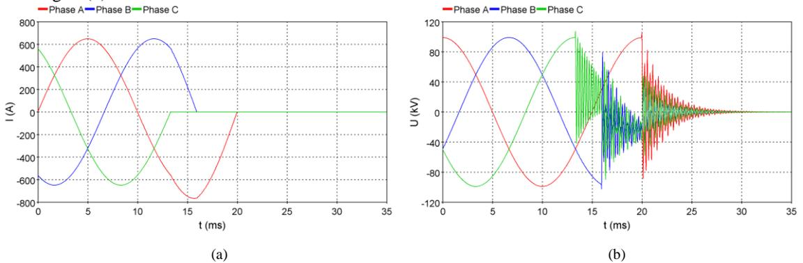
Fig. 9. (a) Shunt reactor currents; (b) shunt reactor overvoltages
