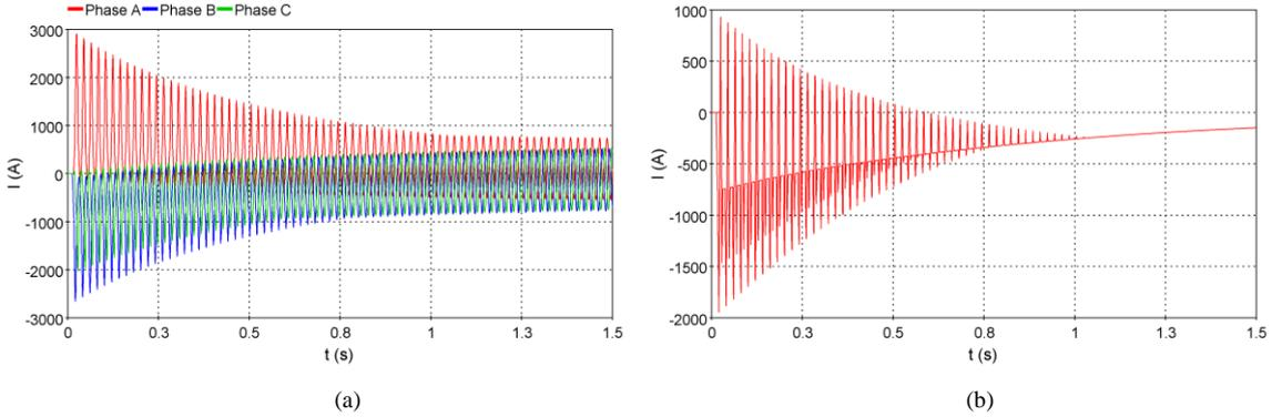
Fig. 6. (a) Inrush currents:  $I_{Amax}=2910.4$  A (4.39 p.u.); (b) zero-sequence current,  $I_{max}=-1948.5$  A (2.94 p.u.)
