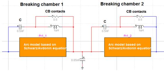
Figure 4. Model of electric arc in EMTP-RV: 400 kV SF<sub>6</sub> circuit breaker with two breaking chambers
