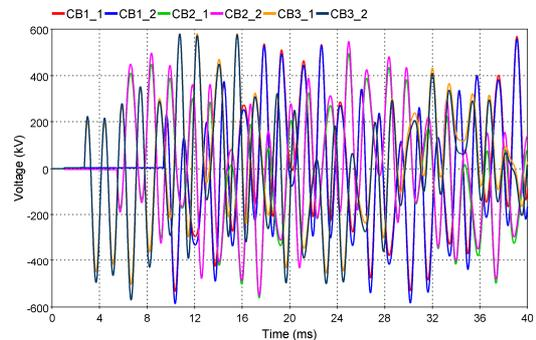
Figure 14. Voltages across breaking chambers (with grading capacitors)
