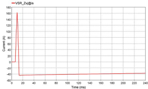
Figure 12. VSR zero-sequence current,  $I_{Zmax} = 162.3$  A
