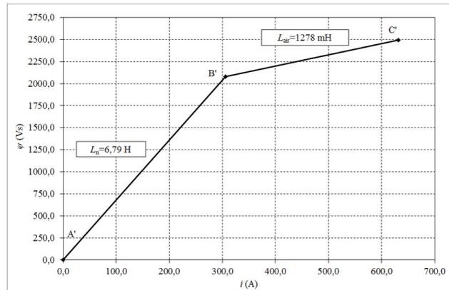
Figure 3. Instantaneous flux-current saturation curve (75 MVar)
