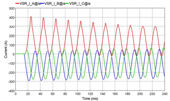
Figure 7. VSR currents:  $I_{Amax}=408.4$  A,  $I_{Bmax}=-295.1$  A,  $I_{Cmax}=-279.1$  A
