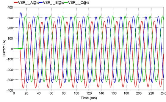
Figure 9. VSR currents:  $I_{Amax} = -381.0$  A,  $I_{Bmax} = 344.4$  A,  $I_{Cmax} = -322.6$  A
