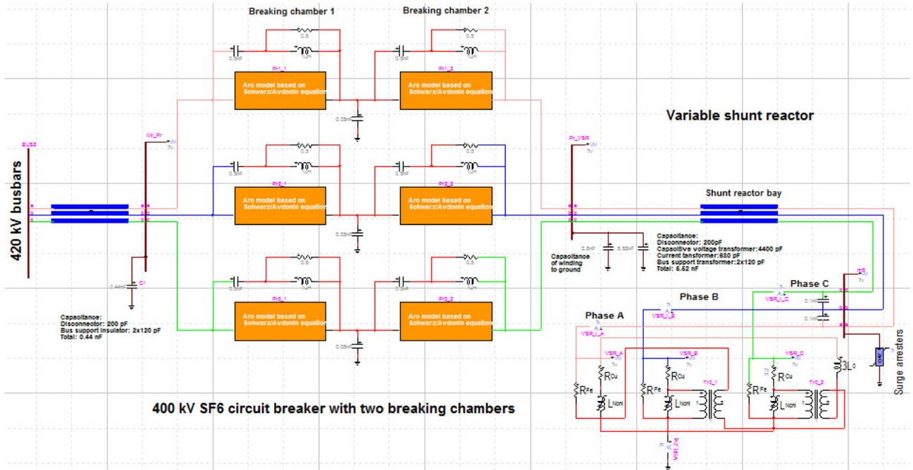
Figure 1. Model of VSR in EMTP-RV
