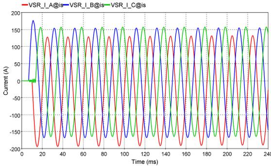
Figure 11. VSR currents:  $I_{Amax} = -193.2$  A,  $I_{Bmax} = 176.9$  A,  $I_{Cmax} = -165.3$  A
