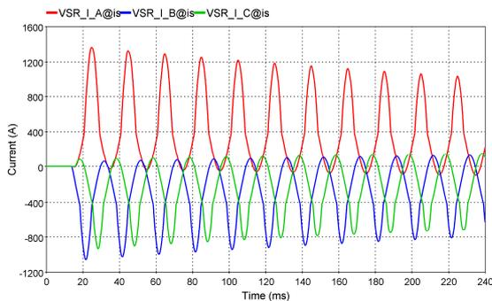
Figure 5. VSR currents:  $I_{Amax}=1362.0$  A,  $I_{Bmax}=-1059.0$  A,  $I_{Cmax}=-936.0$  A
