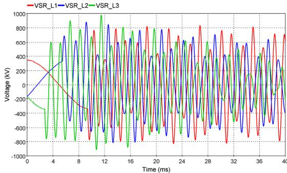
Figure 15. VSR overvoltages:  $U_{Amax}=834.8$  kV,  $U_{Bmax}=880.2$  kV,  $U_{Cmax}=978.9$  kV
