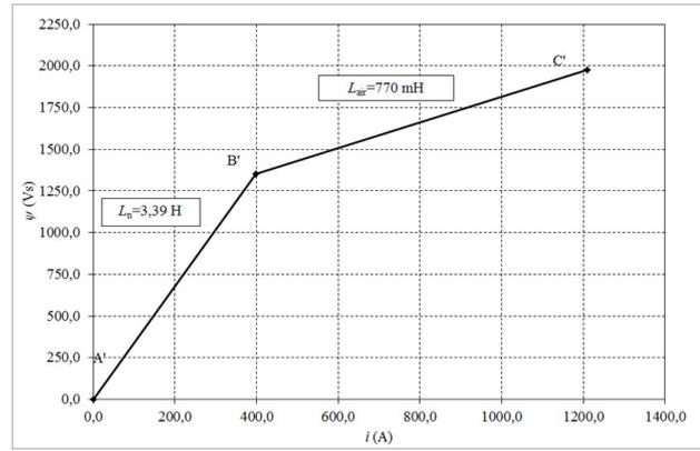
Figure 2. Instantaneous flux-current saturation curve (150 MVar)
