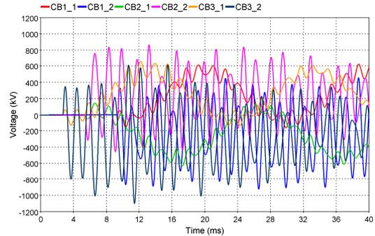
Figure 13. Voltages across breaking chambers (without grading capacitors)
