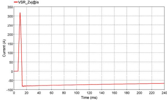
Figure 10. VSR zero-sequence current,  $I_{Zmax} = 315.5$  A
