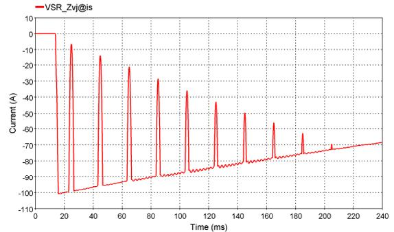
Figure 8. VSR zero-sequence current,  $I_{Zmax}=-100.9$  A
