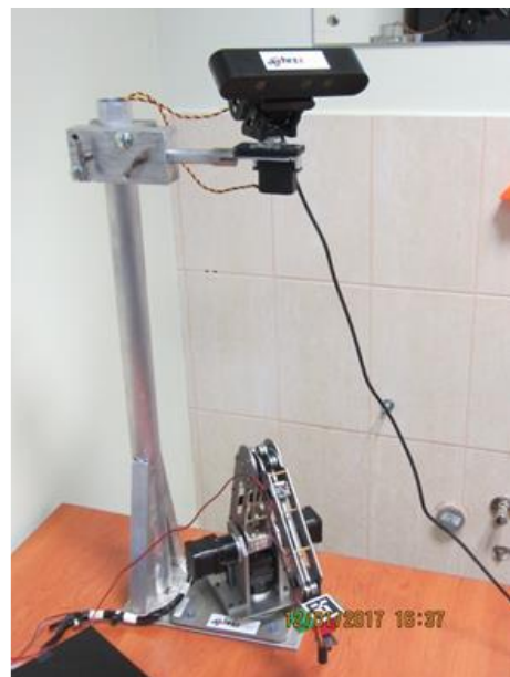
Figure 1. Robot Arm mounted on the stand
