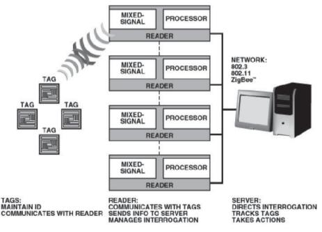
Figure 3 Simplified representation of an RFID system
