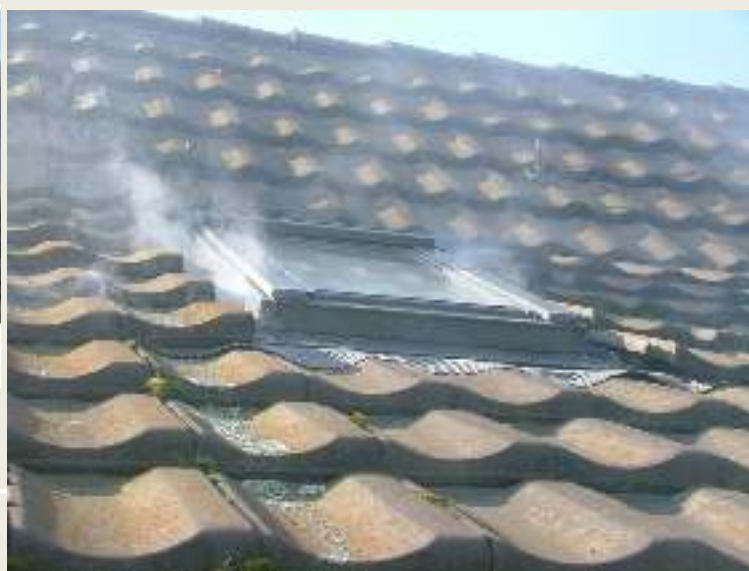
Smoke pressed out by a Blower Door fan to show the roof leaks
