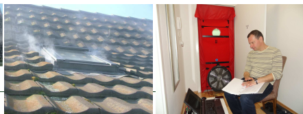
Smoke pressed out by a Blower Door fan to show the roof leaks
