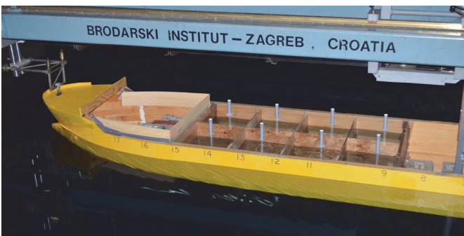
Fig. 6 Towing procedure of the damaged model
