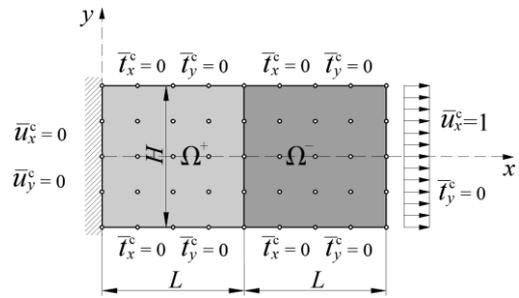
Figure 2: Plate with classical boundary conditions
