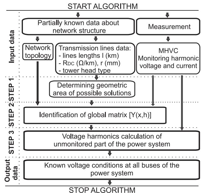
**Fig. 2.** Flowchart of proposed algorithm for estimation of voltage harmonics in unmonitored part of PS.
