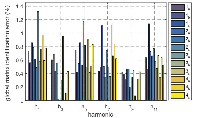
**Fig. 11.** Global matrix  $[Y(x, h)]$  identification error per current harmonics and buses for default accuracy of 0.1%.
