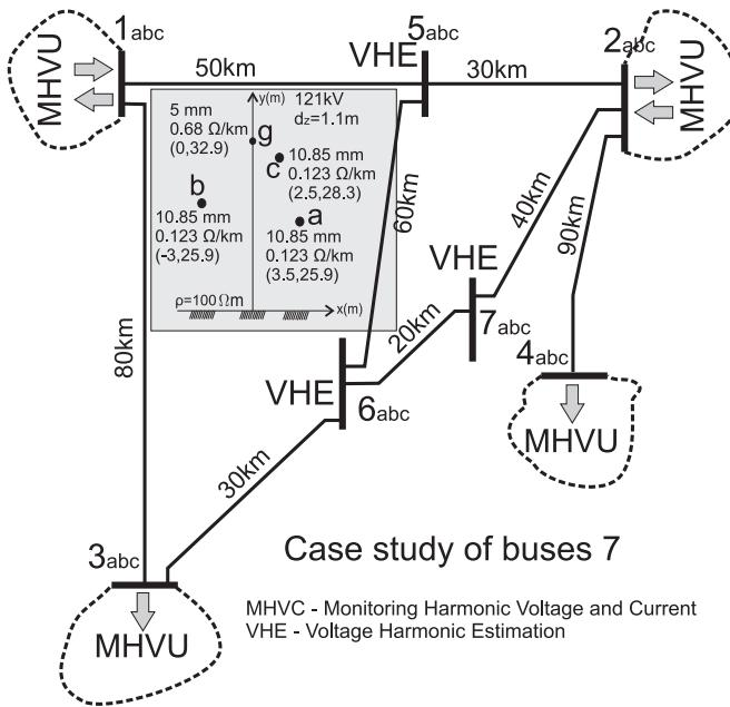
**Fig. 6.** Scheme of analyzed example (case study).
