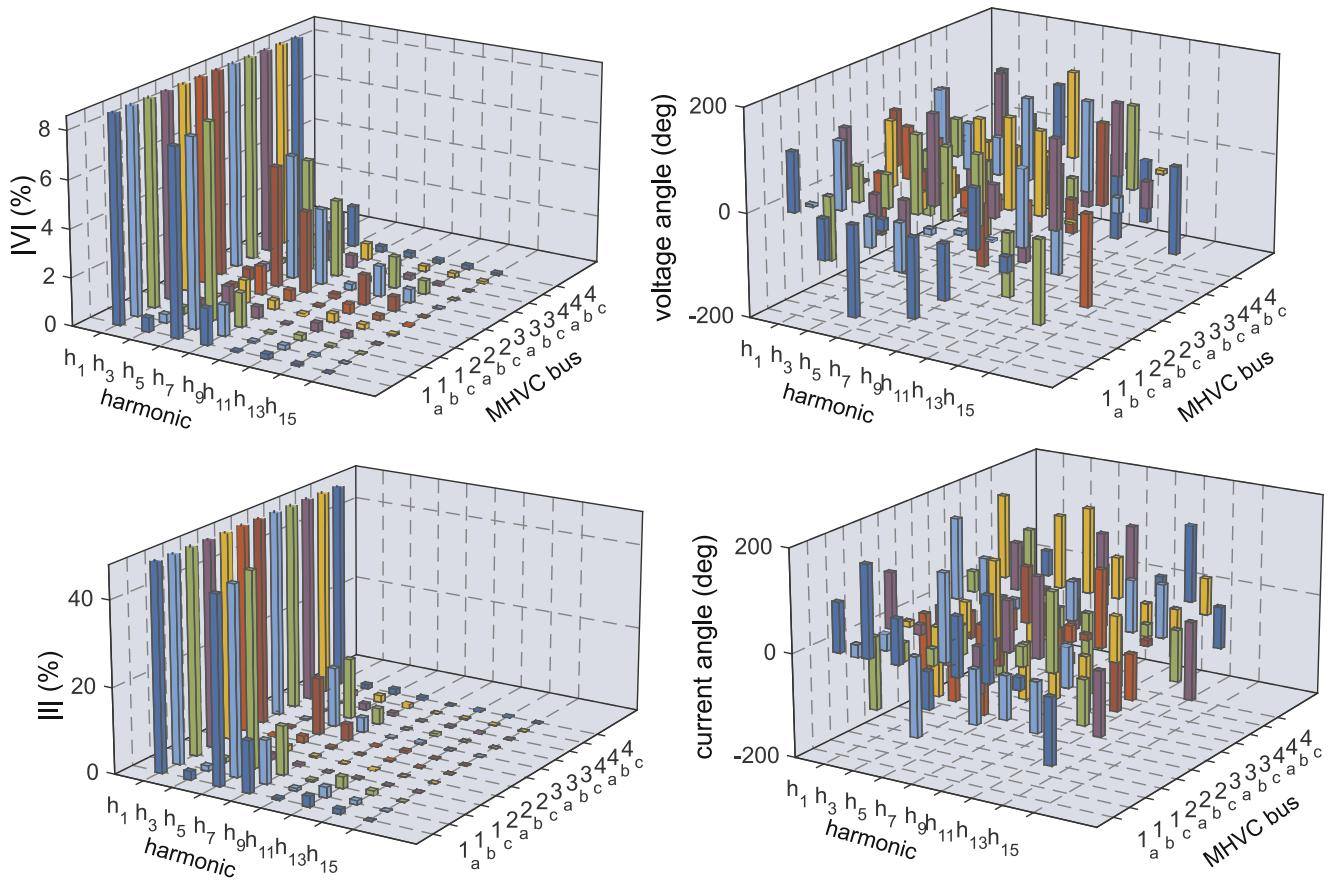
**Fig. 7.** Odd harmonics content (its percentage share compared to fundamental harmonic content) in voltage and current waveform on monitored busses of the PS.
