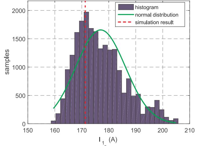
**Fig. 10.** Sample distribution of fundamental current harmonic on bus 1 (phase a) for accuracy of 1%.
