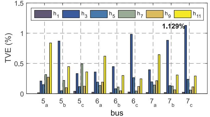
**Fig. 16.** Harmonic estimation error of unmonitored buses.
