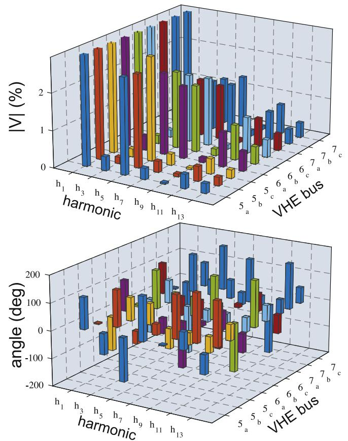
**Fig. 15.** Estimated voltage conditions at unmonitored PS buses.
