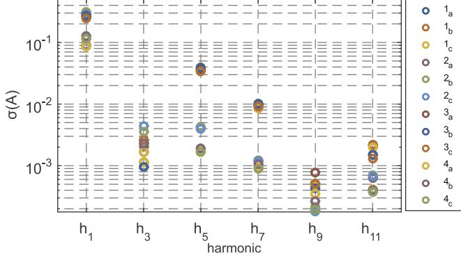
**Fig. 9.** Standard deviation of current harmonics at MHVC buses.
