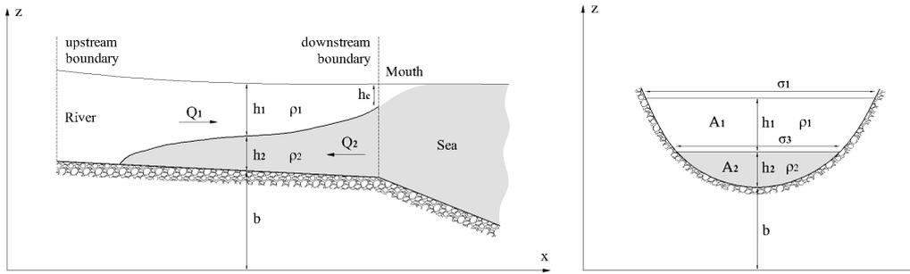
**Fig. 3. Notations for a longitudinal and cross section of the channel**
