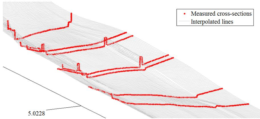
**Fig. 4. Detail of Rječina channel geometry – cross section interpolation**
