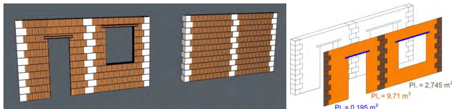
Figure 9: Basic 3D BIM models of bearing walls, one with and one without openings (left) and external surfaces necessary for further cost and time analysis (right)
