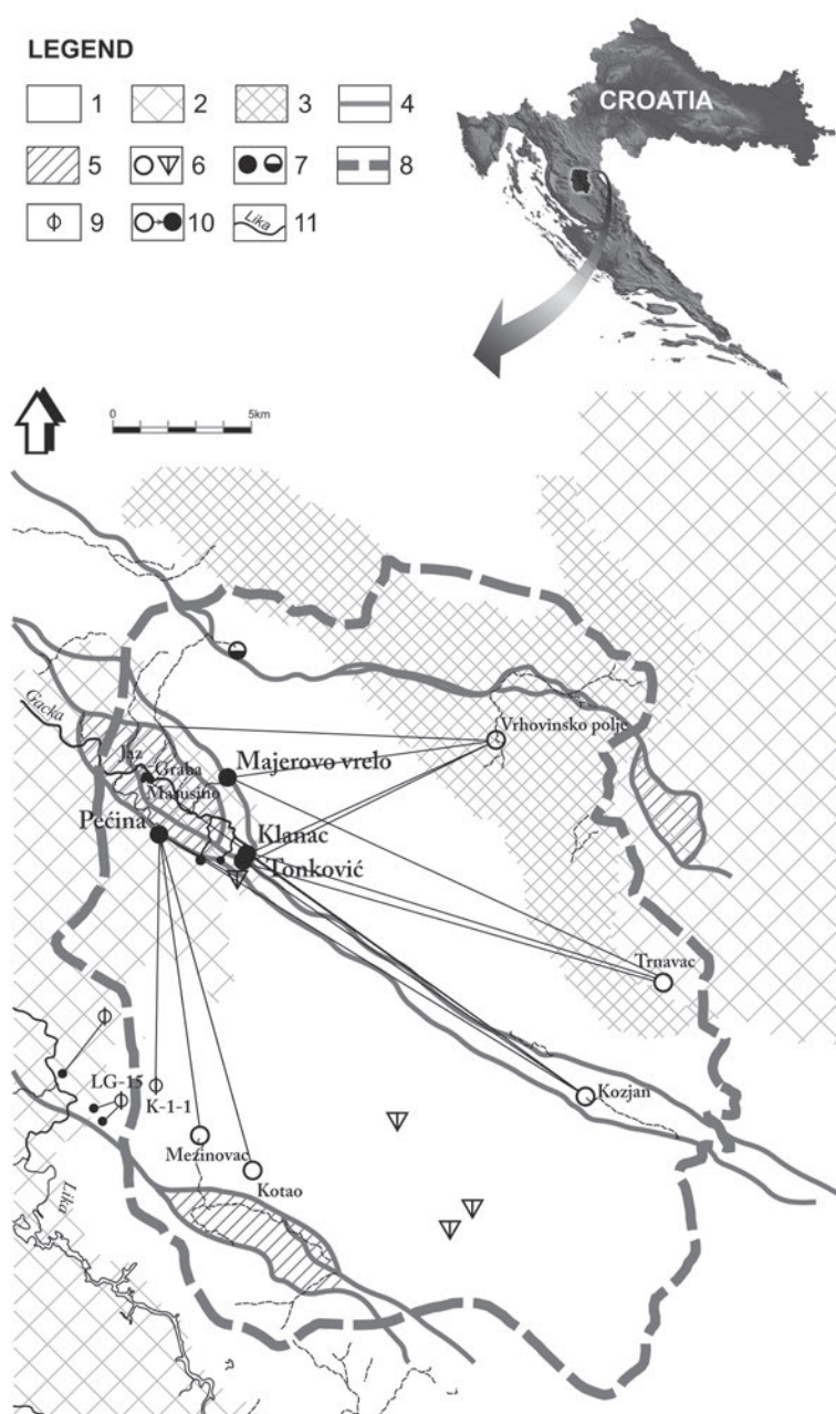
Fig. 21 Schematic hydrogeological map of the study area, showing sampling sites (position of the study area in detail). 1- very permeable rocks, 2- predominantly permeable rocks, 3- predominantly impermeable rocks, 4- most important faults, 5- extension zone, 6- swallow hole (ponor) and vertical cave (pit), 7- spring: permanent and intermittent, 8- groundwater divide, 9- borehole, 10- groundwater connection (tracer test), 11- river, 12- river and rain gauge stations, 13- groundwater velocity determined by tracing tests (cm/s).
